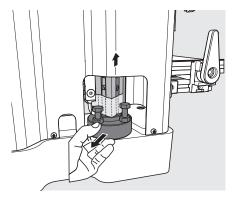
The revolver is located on the back of the machine.
