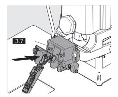
3.7.2) Clipping fitting onto insertion ram (3.7)
