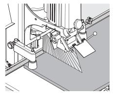
3.7.4) Pushing work piece to the marking line
