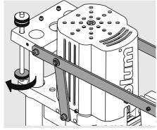
· Completely loosen bottom knurled screw
