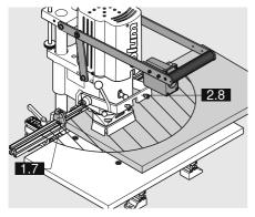
**3.1.7) Placing carcase side on the work table and pushing up against the stop** (See point 2.1.9)
