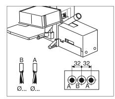
4.3.9) H drilling head: M65.26XX horizontal drilling unit for dowel connections, cabinet connector screws and furniture connectors
