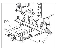
2.1.4) Setting up and securing machine to a suitable table
