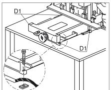
• Secure the machine to the work top using the fixing screws (D1)
