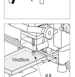
Make vertical drilling (8 mm) in the sample board (approx.10 cm x 20 cm) using the desired drilling distance 2.
