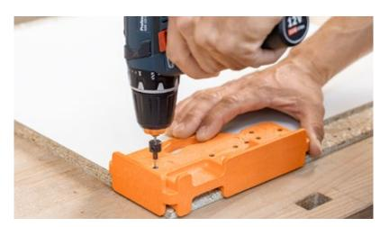
Holes must be drilled with utmost precision. Our drilling templates make it easy to mark and pre-drill the fixing positions for cabinet profiles, so that components are prepared for installation in no time.
