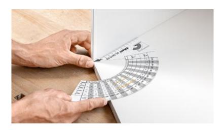
When it comes to mounting fronts, we have further assembly devices in our range. These include drilling templates for hinges which ensure that the drilling positions on the front match precisely those on the cabinet. As a result, hinges work perfectly, doors close softly and gaps are beautifully aligned.
