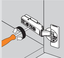
On non-cam mounting plates, loosen screws, adjust door and retighten screws.
